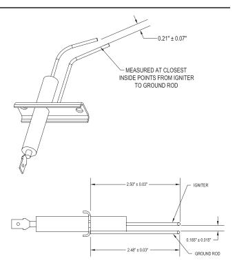
Figure 30. Direct Spark Igniter.
